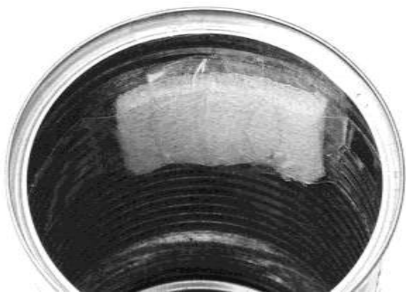
Figure 5-26 Fitting the diffuser
