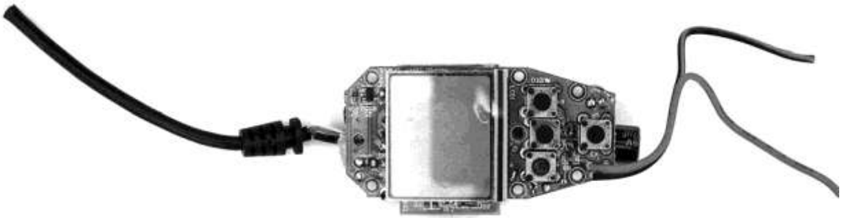
Figure9-11 FM transmitter with leads trimmed
