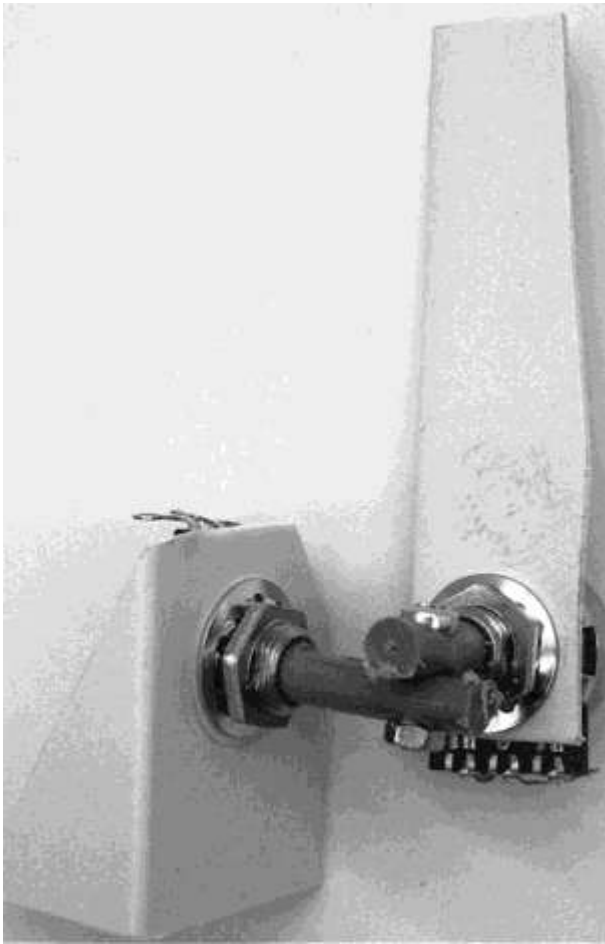
Figure 4-6 The variable resistors attached to each other
