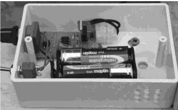
Figure 8-32 The motor controller and batteries boxed
