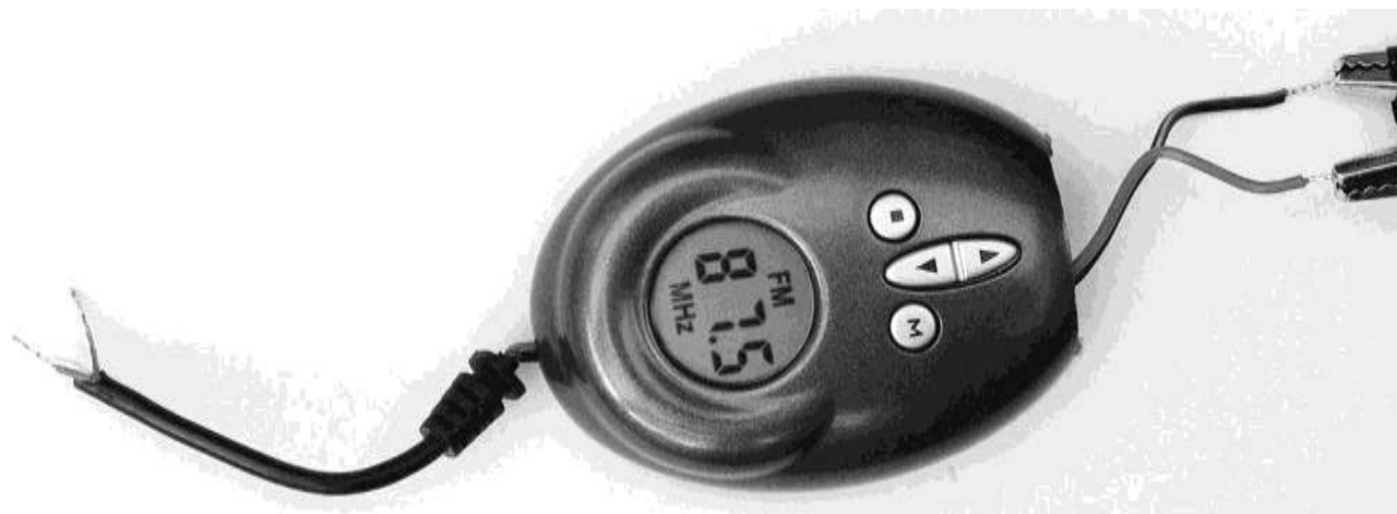
Figure9-12 FM transmitter reduced to basics
