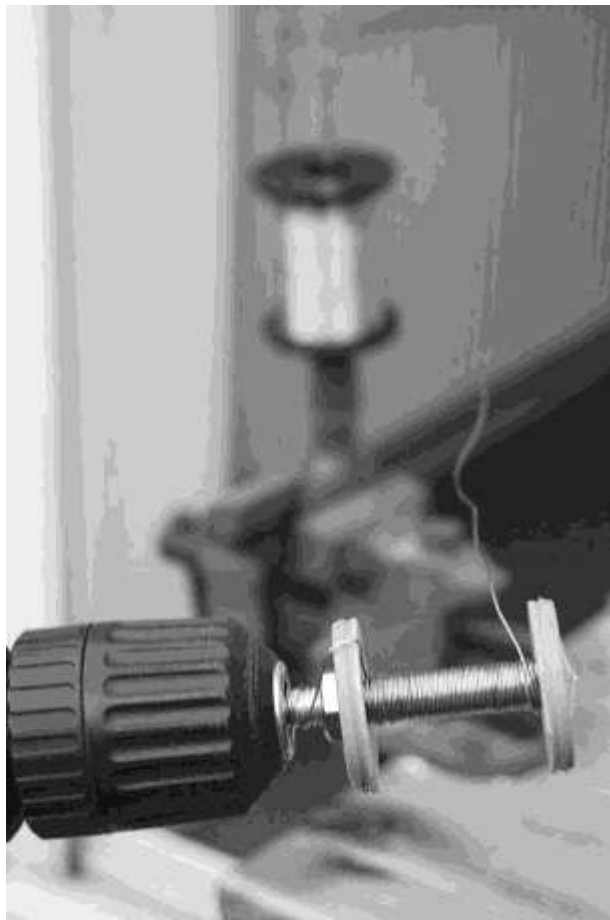
Figure 13-4 Winding using an electric drill
