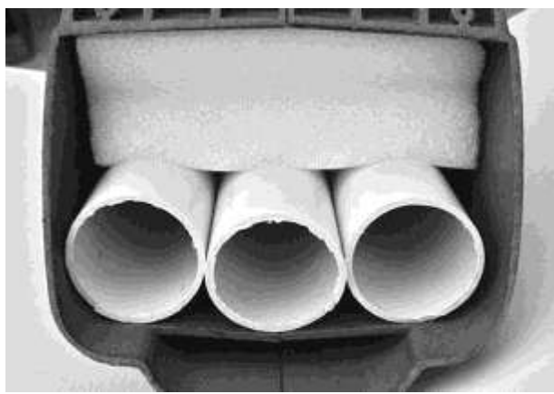
Figure3-8 Pipes in place at the nozzle end
