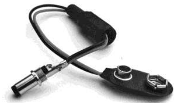
Figure 8-23 The battery clip for the LED unit
