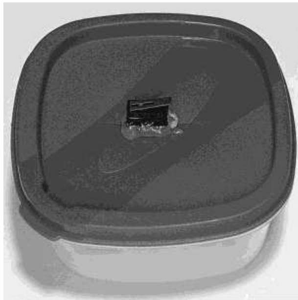
Figure 11-8 The micro-switch attached to the box lid
