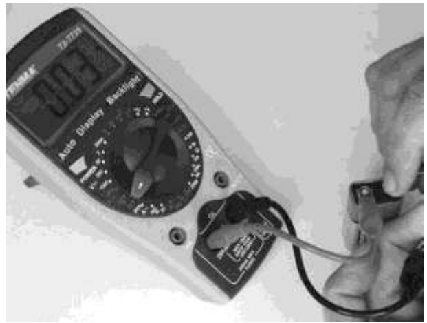
Figure A-8 Measuring current
