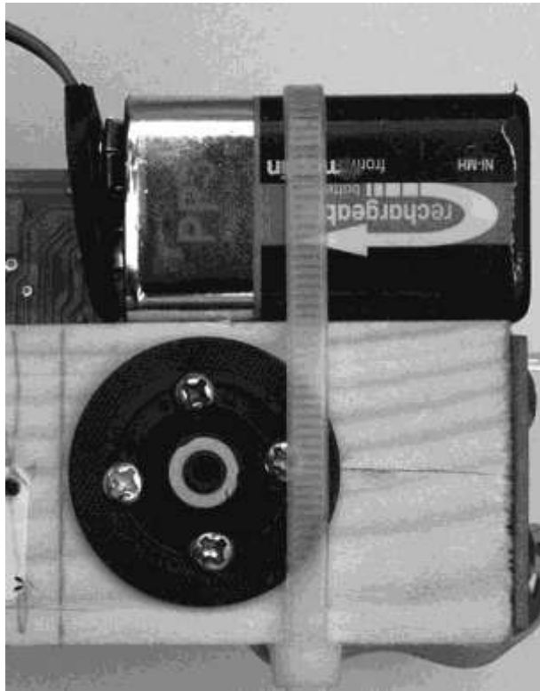
Figure 8-33 Attaching the arm to the motor
