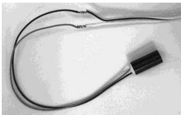
Figure 7-9 Attaching the laser to the cable
