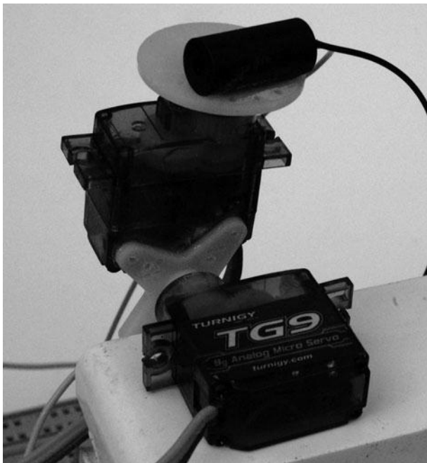
Figure 8-15 Servo and laser assembly.
