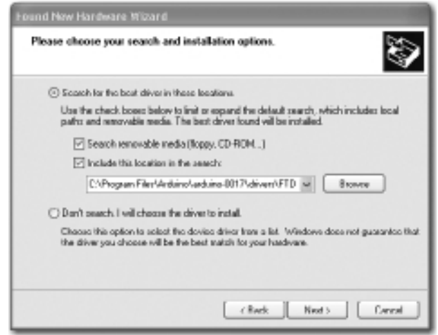
Figure 1-7 Setting the location of the USB drivers.
