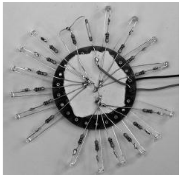
Figure 9-14 Bottom side of Lilypad board.
