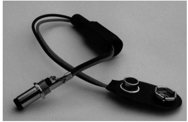
Figure 4-8 Creating a battery lead.
