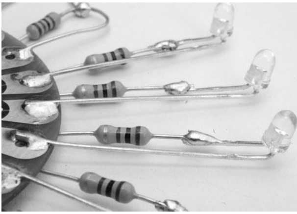
Figure 9-13 Close-up of LED attached to a resistor.
