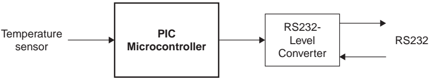
Figure 5.118 Block diagram of Project 26
