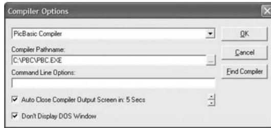
Figure 3.21 Configuring CodeDesigner Lite for the PicBasic compiler
