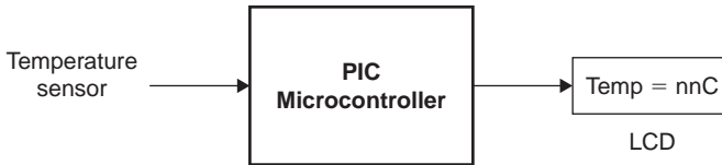
Figure 5.108 Block diagram of Project 24
