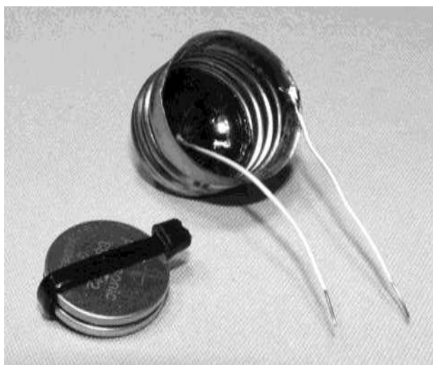
Figure 8-5 Wires soldered to the bulb base
