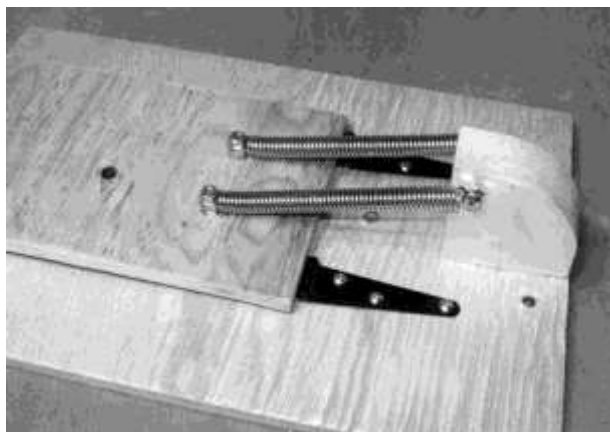
Figure 11-5 Launch springs in the loaded position
