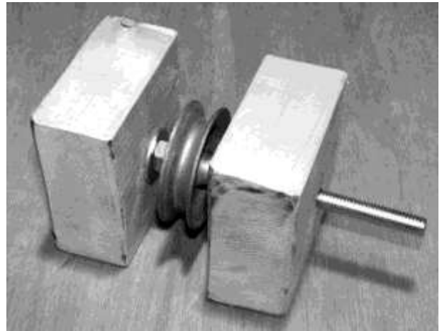
Figure 10-3 Axle support blocks made from pieces of a 2 \times 4 wood
