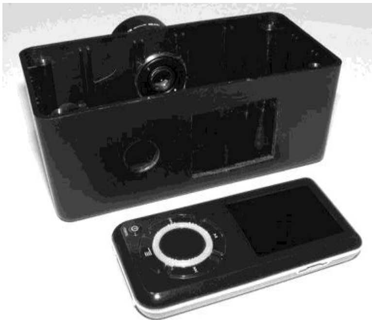
Figure 8-20 Enclosure holes cut for the video player
