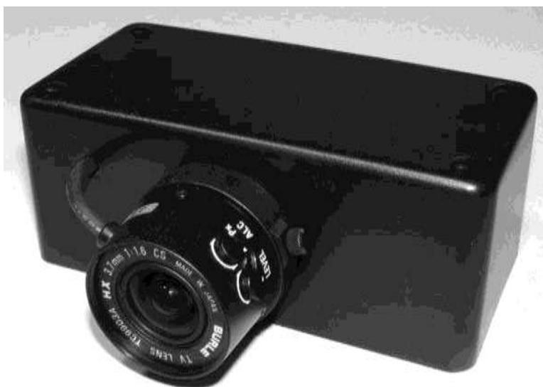
Figure 8-19 Mounting the lens to the enclosure
