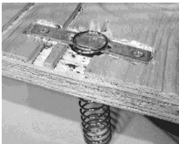
Figure 3-24 The spring is secured to the base
