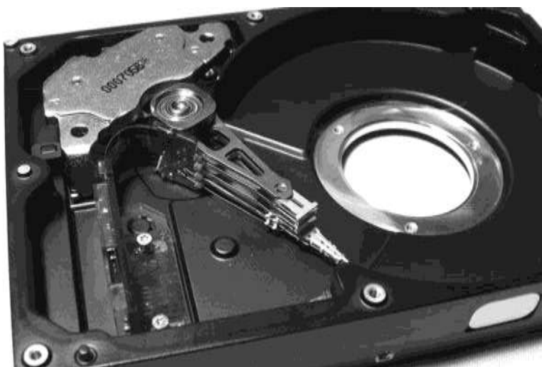
Figure 4-23 Only the arm mechanics remain
