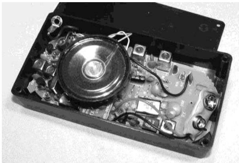
Figure 9-6 Re-fitting the receiver in a smaller box
