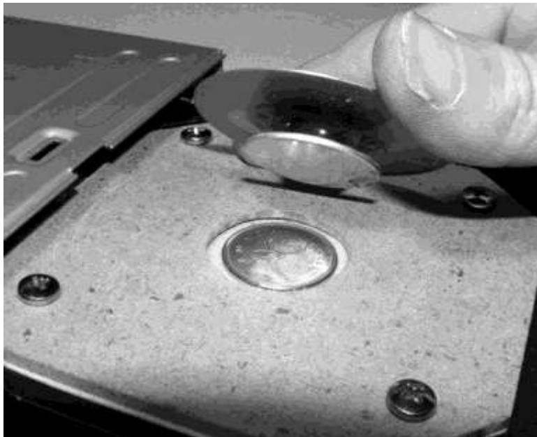
Figure 8-14 Magnet lifts the slug not the quarter
