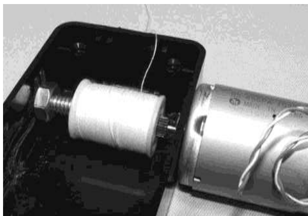
Figure 3-17 Towing mechanics completed
