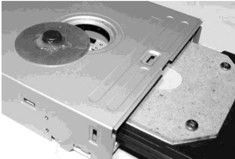
Figure 8-13 Magnet glued to the round lid
