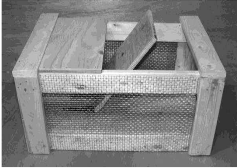
Figure 11-9 The cage lid is also a launch-pad brake
