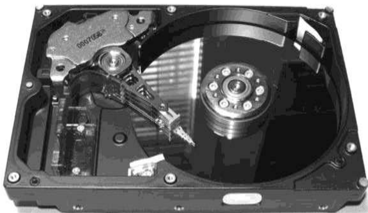
Figure 4-22 Inside a typical hard disk drive
