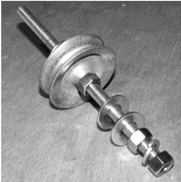
Figure 10-2 Bolts hold the pulley and trolley in place the pulley to the axle and the support block to keep the bolt from rubbing against the wood. The axle hole should also be drilled a little larger than the diameter of the axle (threaded rod) so it can turn freely in the hole with little friction.
