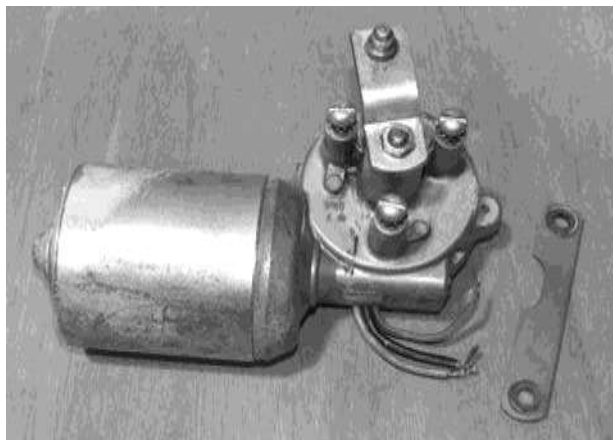
Figure 10-23 The bare wiper motor cleaned and tested
