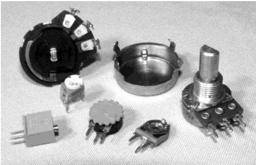
Figure 1-7 Common variable resistors
