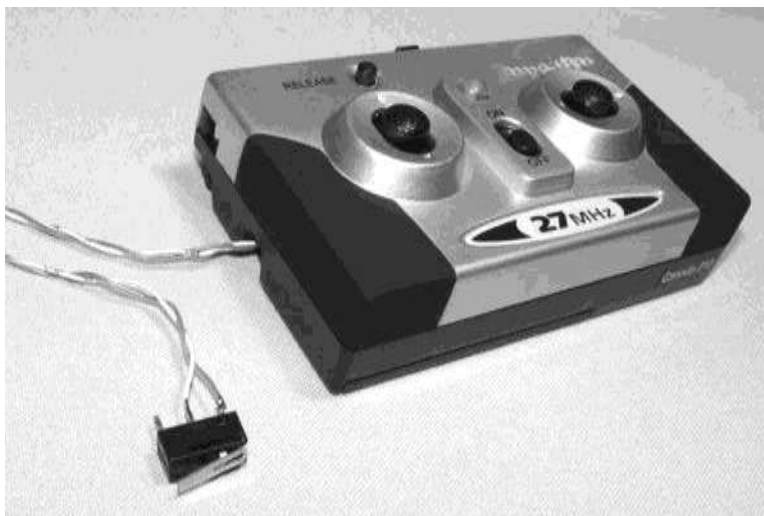
Figure 9-14 Remote-control transmitter and microswitch
