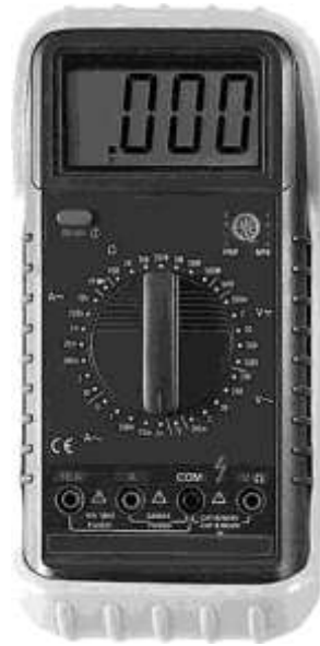
Figure 1-4 A basic multi-meter for electronics work
