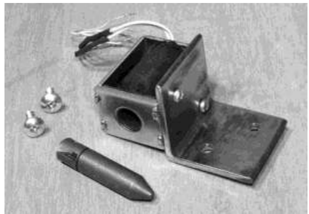
Figure 11-13 An electromagnetic solenoid and plunger
