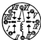
Fig. 3.2. Schema electric  a unui cartu  vibrator.
