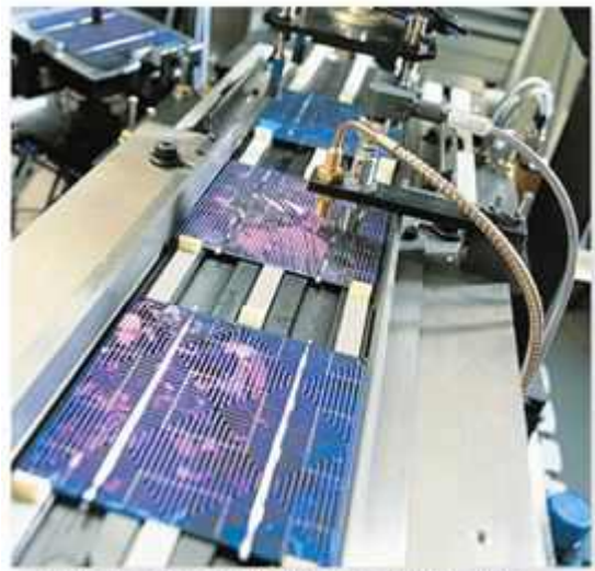
Printing of Photowatt's front-side PV cells.
