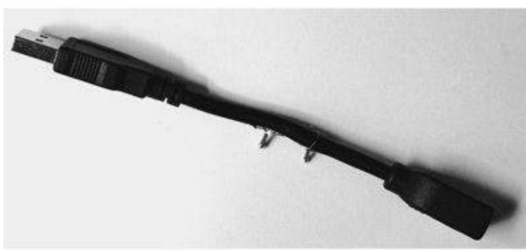
Figure 2-18 Making a USB nonpowered lead
