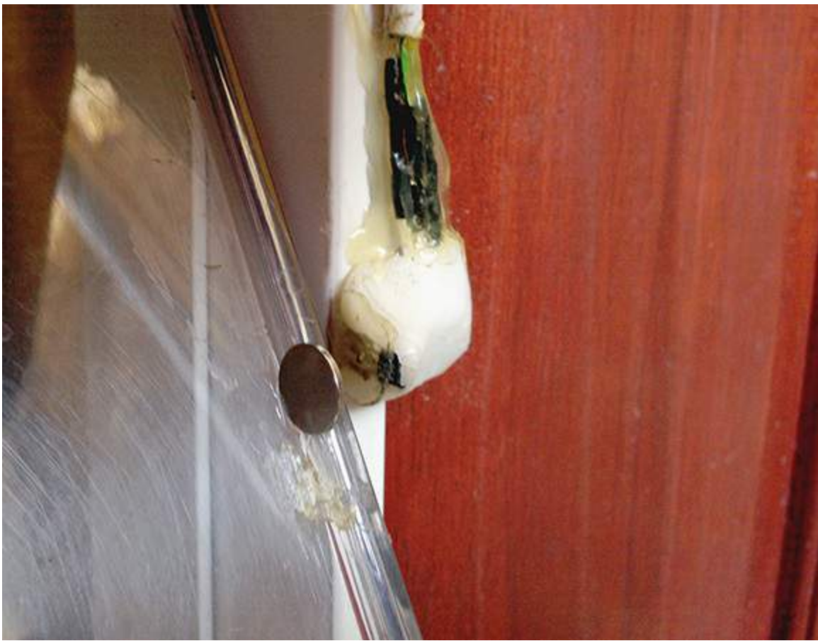
Figure 11-10: Mounting your sensors and magnets.
