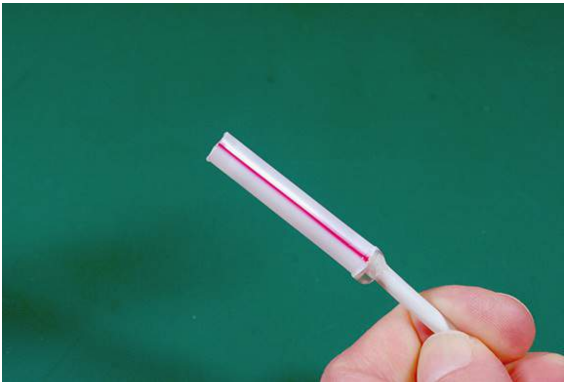
Figure 12-10: Finishing up your sensors for a watertight seal.
