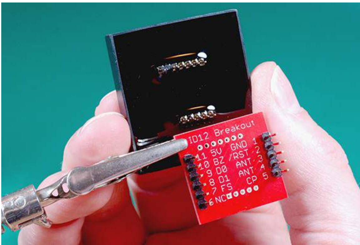
Figure 9-3: The SparkFun breakout board is keyed to fit the ID Innovations readers.
