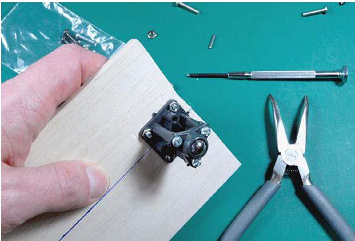
Figure 14-9: Mounting the ball caster.
