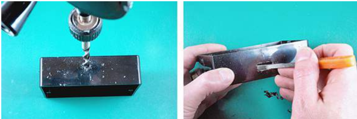
Figure 15-10: Drilling the hole for your power switch.
