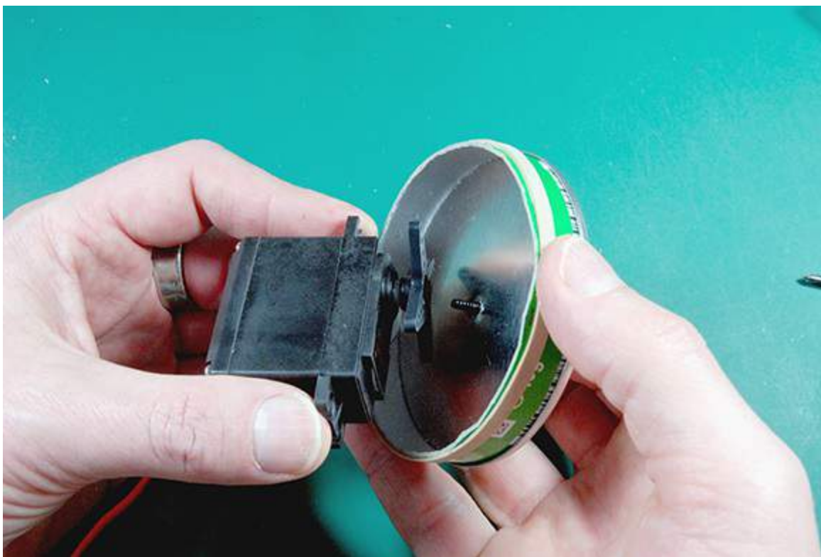
Figure 14-12: Mounting your wheels to the servo motors.
