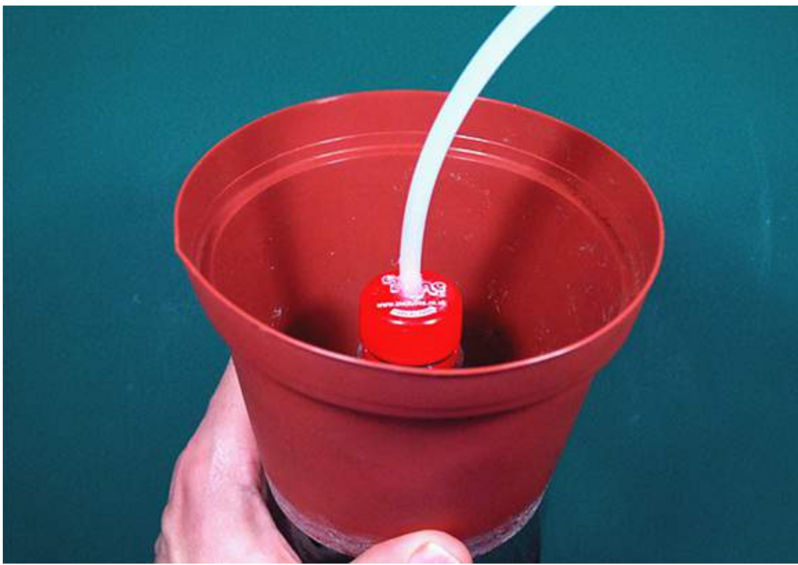
Figure 10-12: Fitting the reservoir onto the base.
