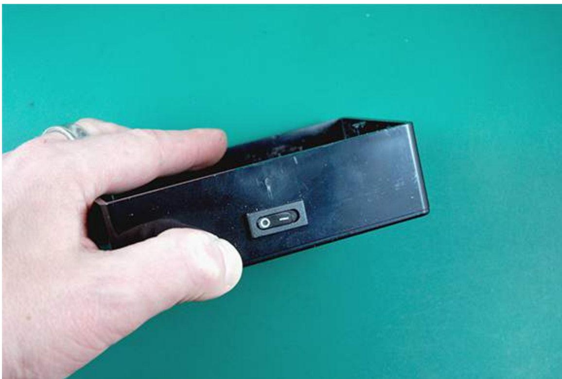
Figure 15-10: Drilling the hole for your power switch.
