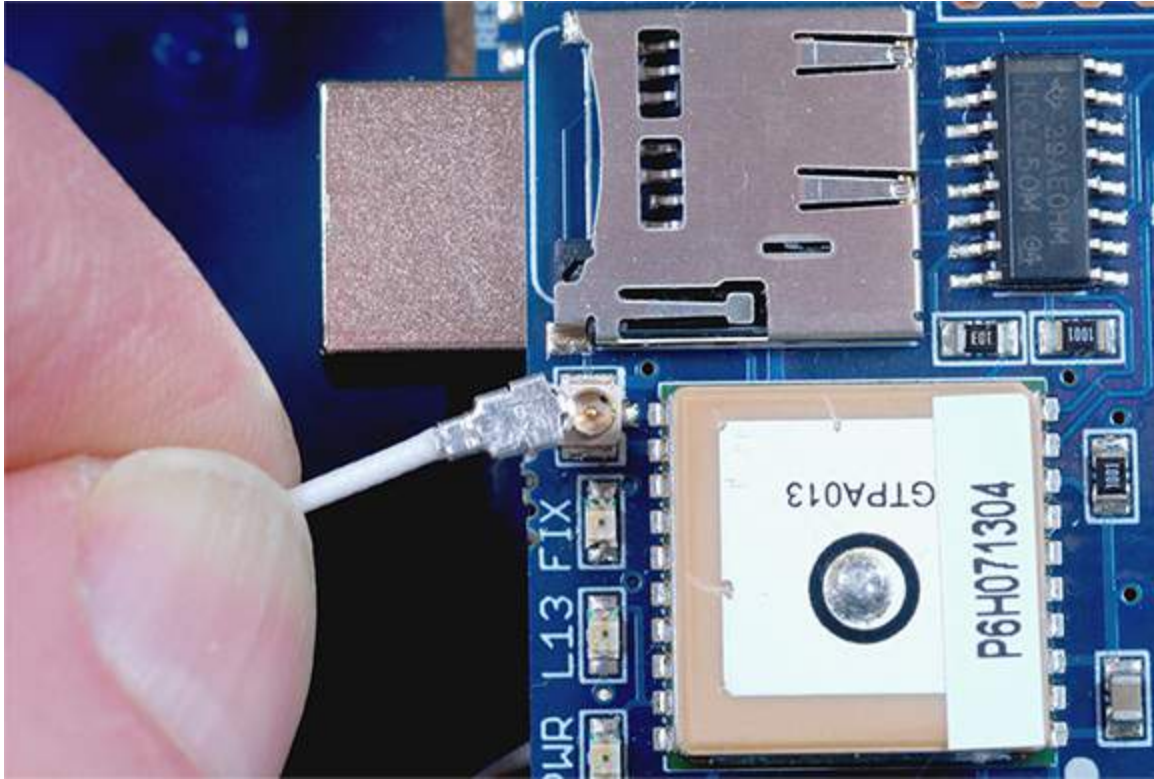
Figure 13-17: Connecting the optional external antenna adapter.
