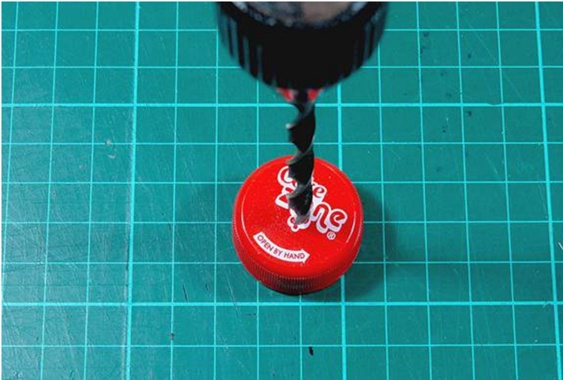
Figure 10-10: Drilling a hole for your supply line.
