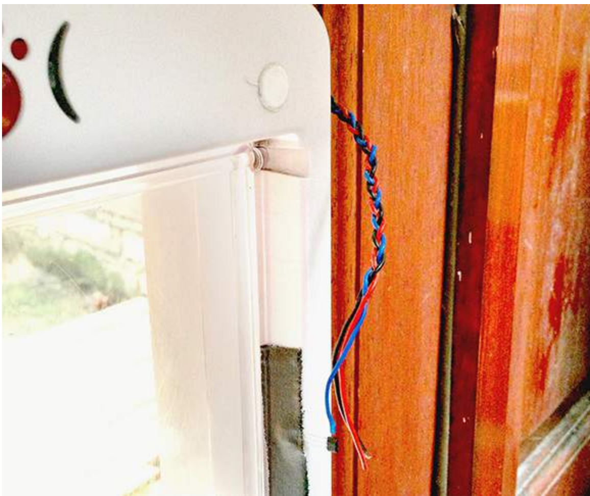
Figure 11-8: Taping your sensors in place to estimate the signaling wire length.
