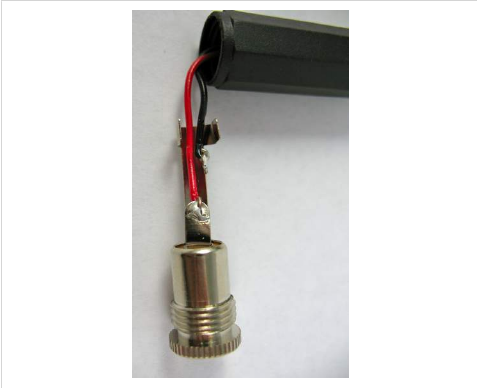
Figure 5-5. Power jack with wiring soldered in place
