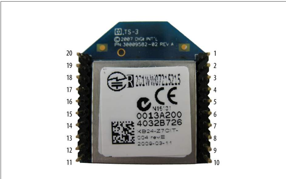
Figure 1-12. XBee physical pin numbering, back view
