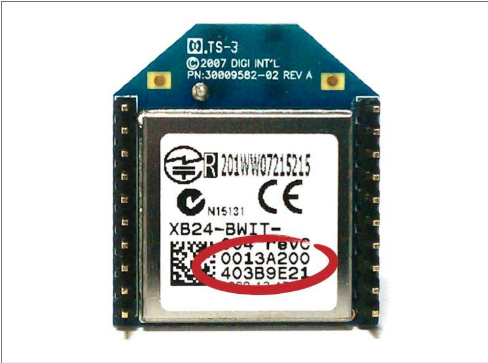
Figure 2-22. Back of XBee showing 64-bit address
