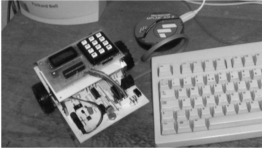
Figure 7.21 ICD 2 connected to a Derbot AGV
