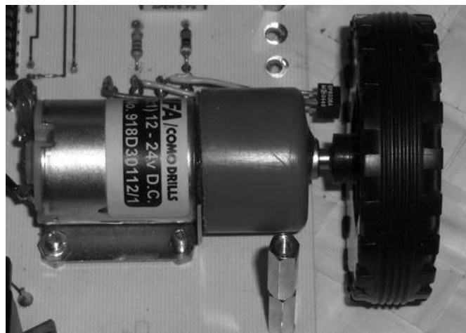
Figure 8.22 A Derbot geared motor MFA/Como RE280/1
