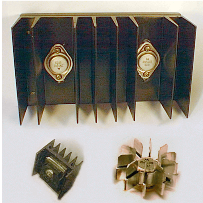
Fig. 1. Examples of heat sinks. Clockwise from top: power supply heat sink with two TO-3 case-style BJTs; pressure-fit heat sink over TO-5 case-style BJT; heat sink with TO-220 case-style BJT.
