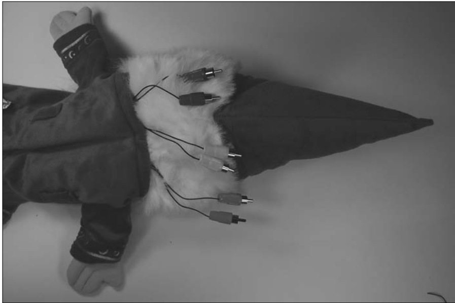
Figure 7-18: Place tactile switches in the puppet.
