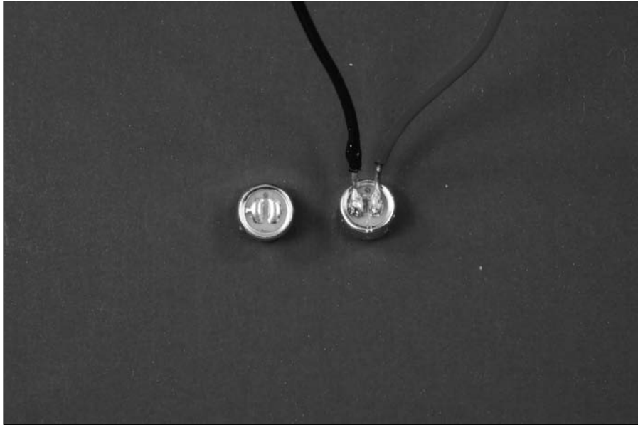
Figure 4-14: Soldering to flat contact pads.
