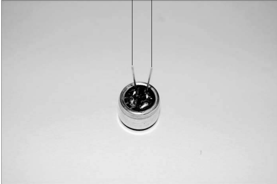
Figure 14-12: Identifying the micro- phone leads to which you will solder wires.
