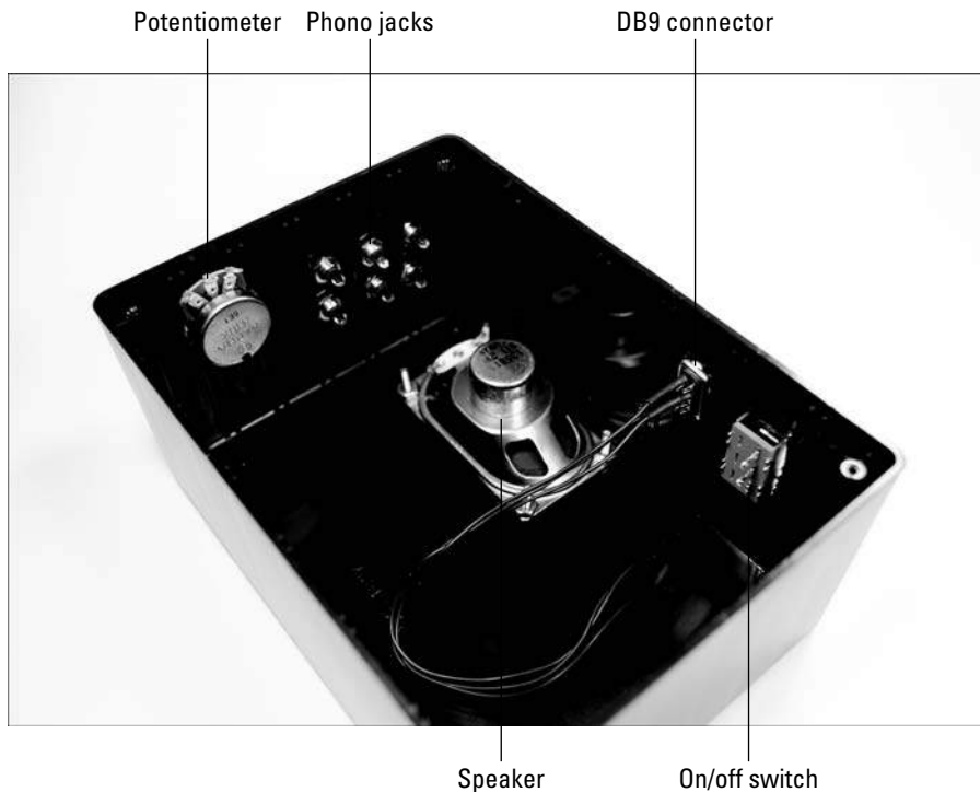
Figure 7-11: Mount components on the box.
