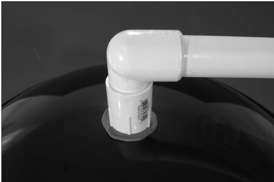
Figure 6-11: Fittings assembled on the parabolic dish.
