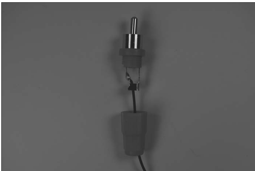
Figure 7-17: Solder wires to phono plugs.
