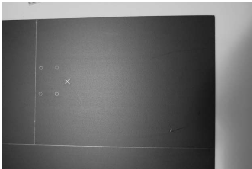
Figure 11-34: Mark the base for cutting and drilling.
