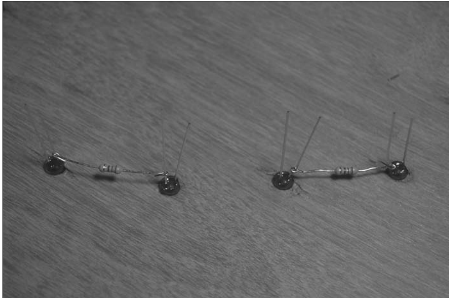
Figure 10-16: Attach resistors to LEDs.
