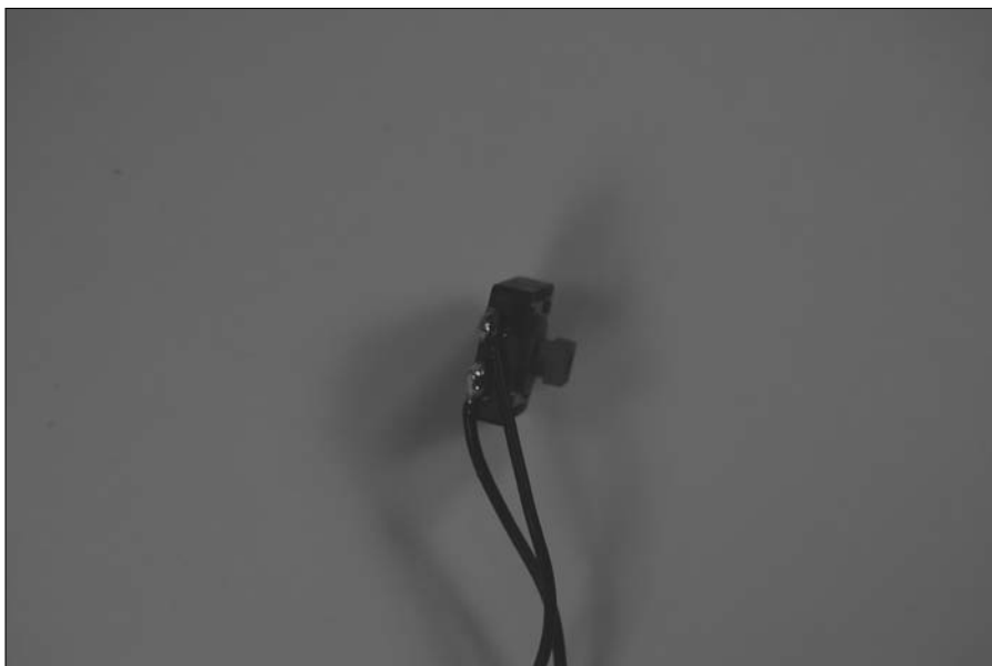
Figure 7-16: Solder wires to tactile switches.
