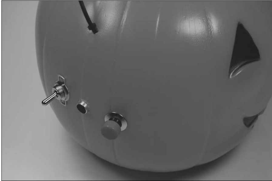
Figure 9-29: Switches and microphone mounted on pumpkin.
