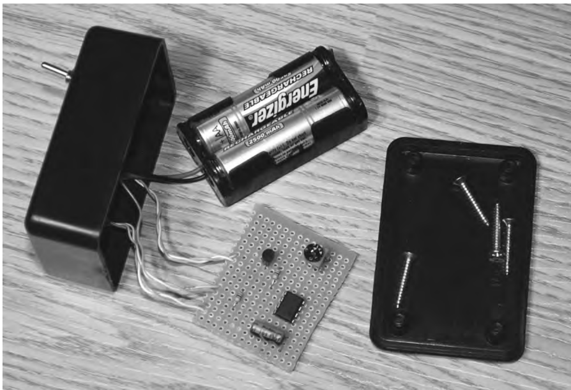
Figure 15-8 Putting together the oscillator unit.
