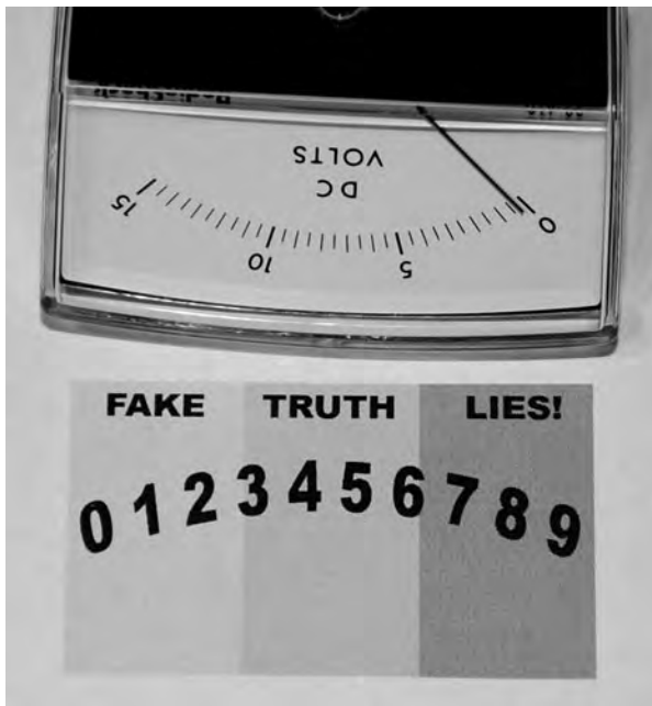
Figure 6-4 Making a replacement readout plate.
