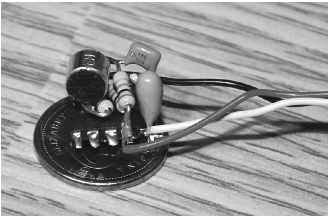
Figure 4-6 Building a circuit without a circuit board.
