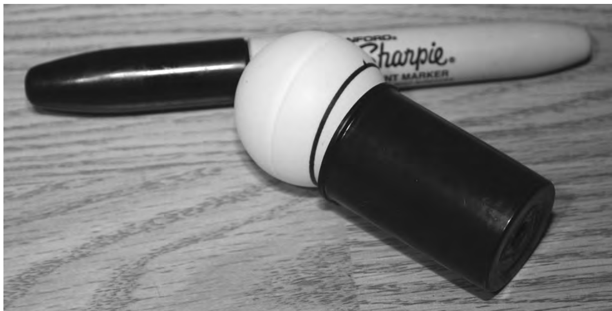
Figure 18-7 Making a diffuser tube for the goggles.
