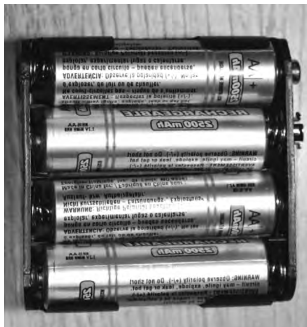
Figure 2-7 Six volts from four batteries.
