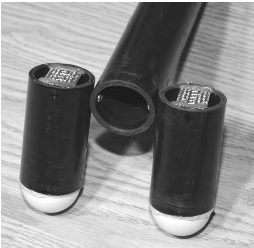
Figure 14-11 Adding a support tube for tripod mounting.
