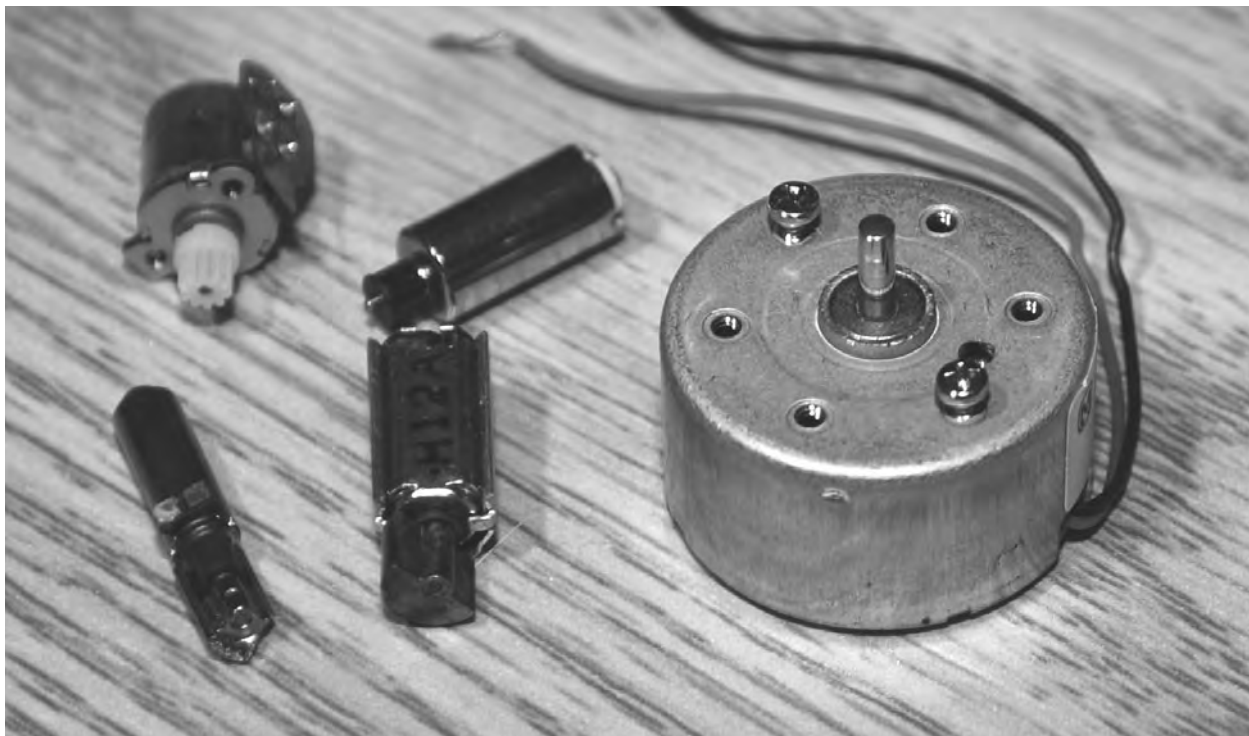
Figure 9-3 Small dc motors that can make vibrations.
