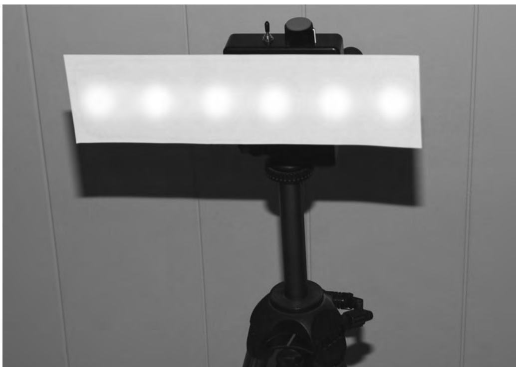
Figure 17-6 Diffuser screen lit by the LEDs.
