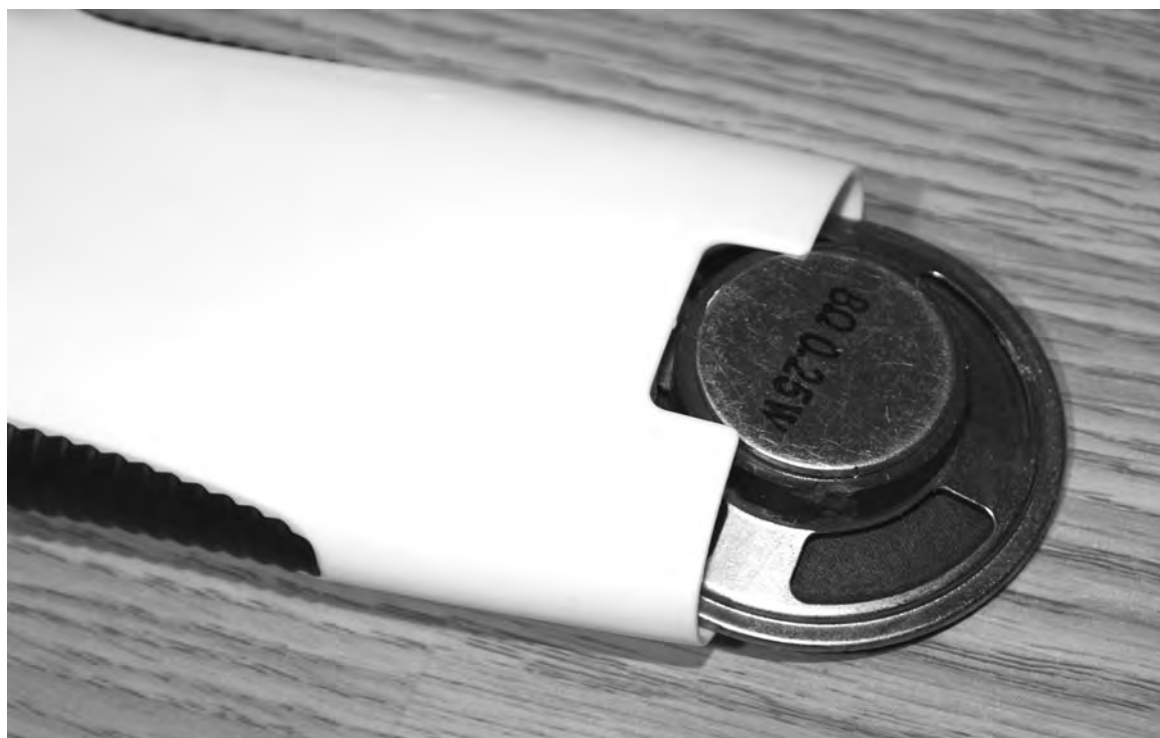
Figure 10-16 Making a simple pillow speaker.
