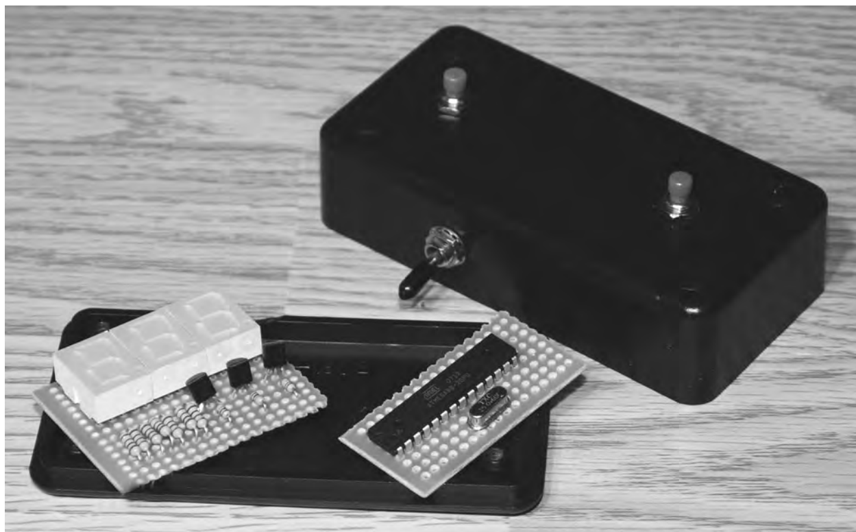
Figure 16-4 Deciding on a cabinet and board layout.
