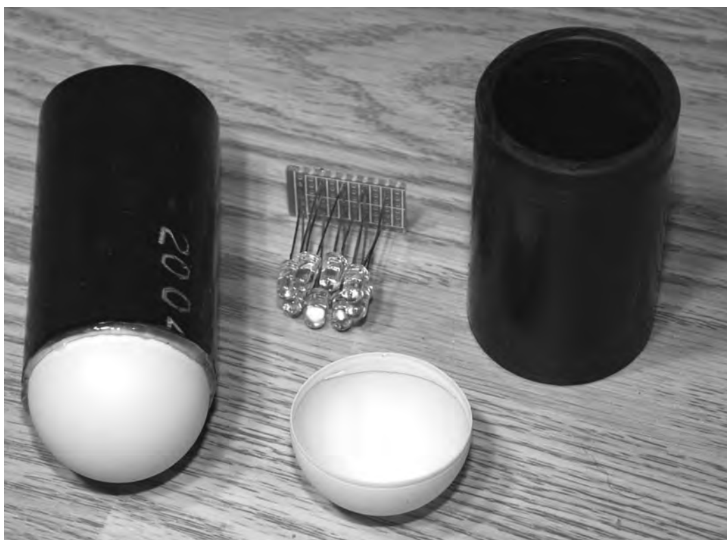
Figure 14-9 Making housing for the components.
