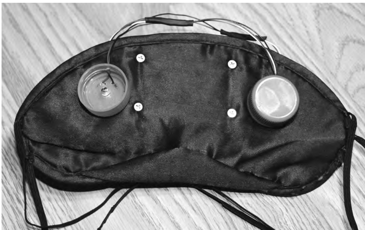
Figure 12-7 Installing the hardware onto the sleep mask.
