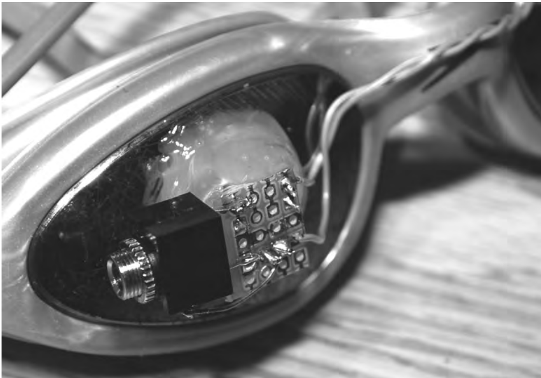
Figure 15-7 Wiring the LEDs for external access.
