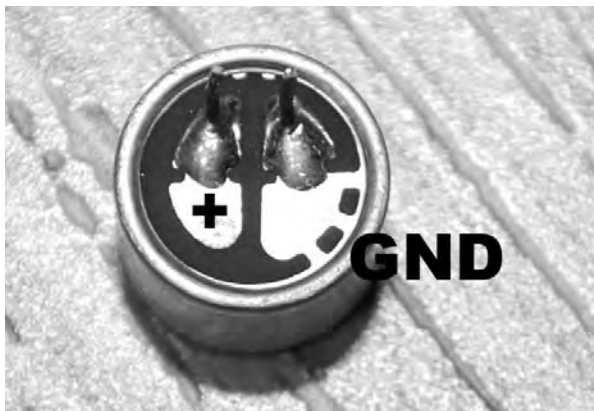
Figure 4-3 Electret microphones are polarized.
