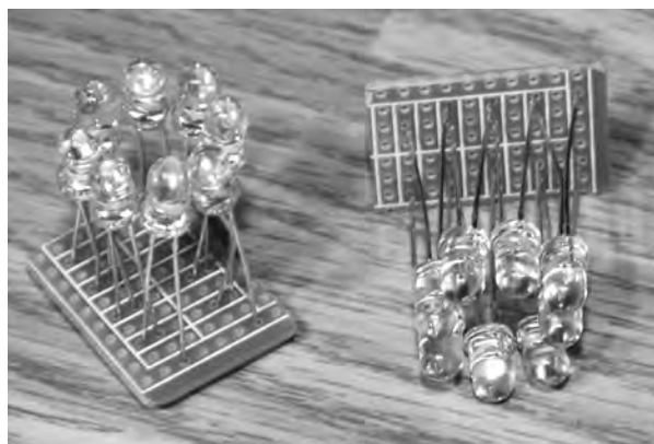
Figure 14-8 Soldering the LED clusters to a perf board.
