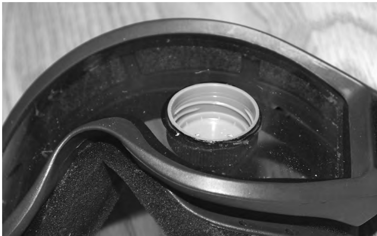
Figure 11-9 Inserting the cap through the lens hole.
