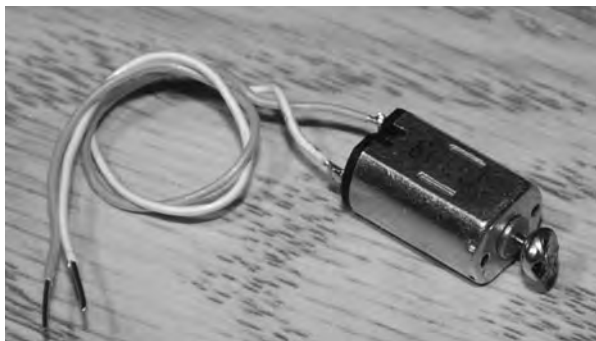
Figure 9-5 Motor with counterweight attached.
