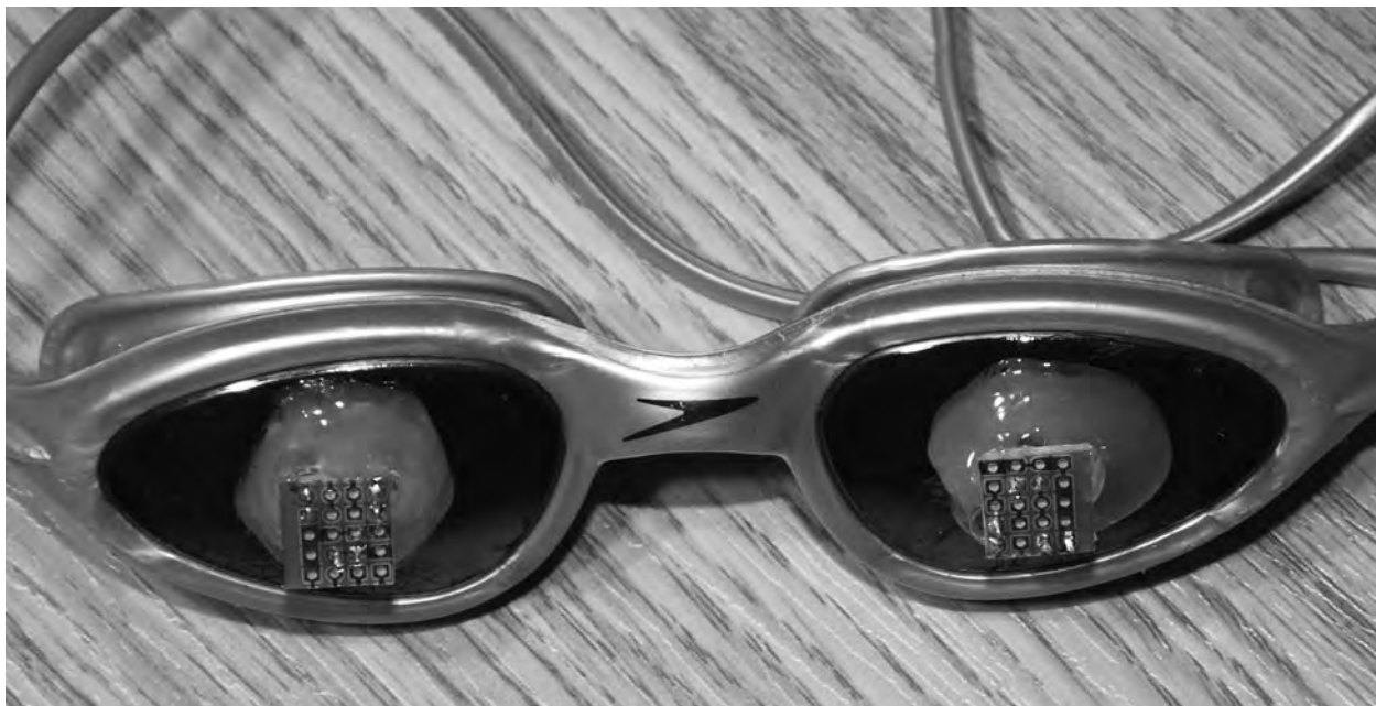
Figure 15-6 Mounting the LEDs to the goggles.
