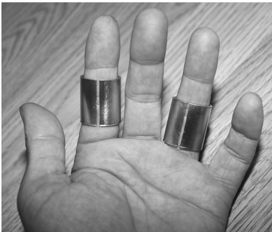
Figure 1-9 Test-fitting the two finger probes.
