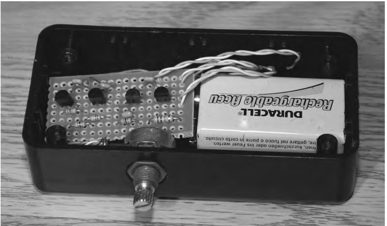
Figure 1-7 Test-fitting the circuit board.
