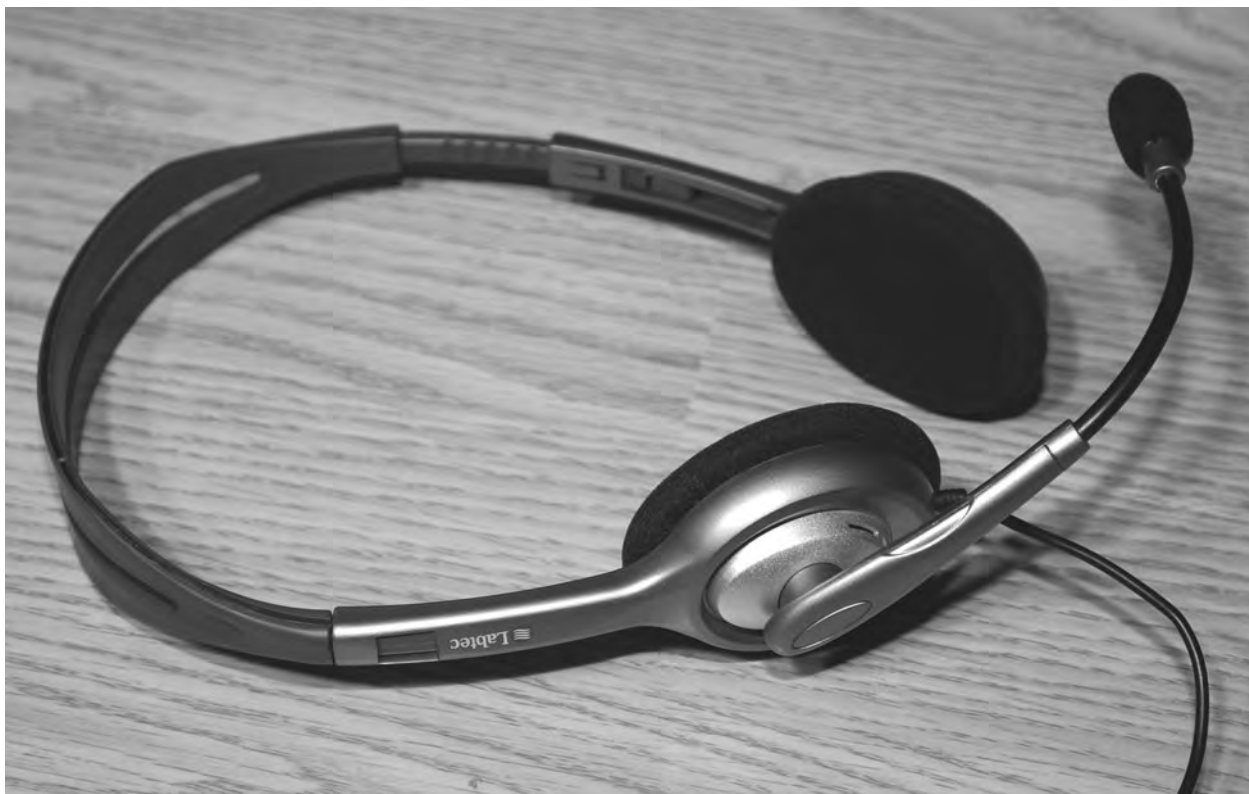
Figure 4-4 A headset containing an electret microphone.
