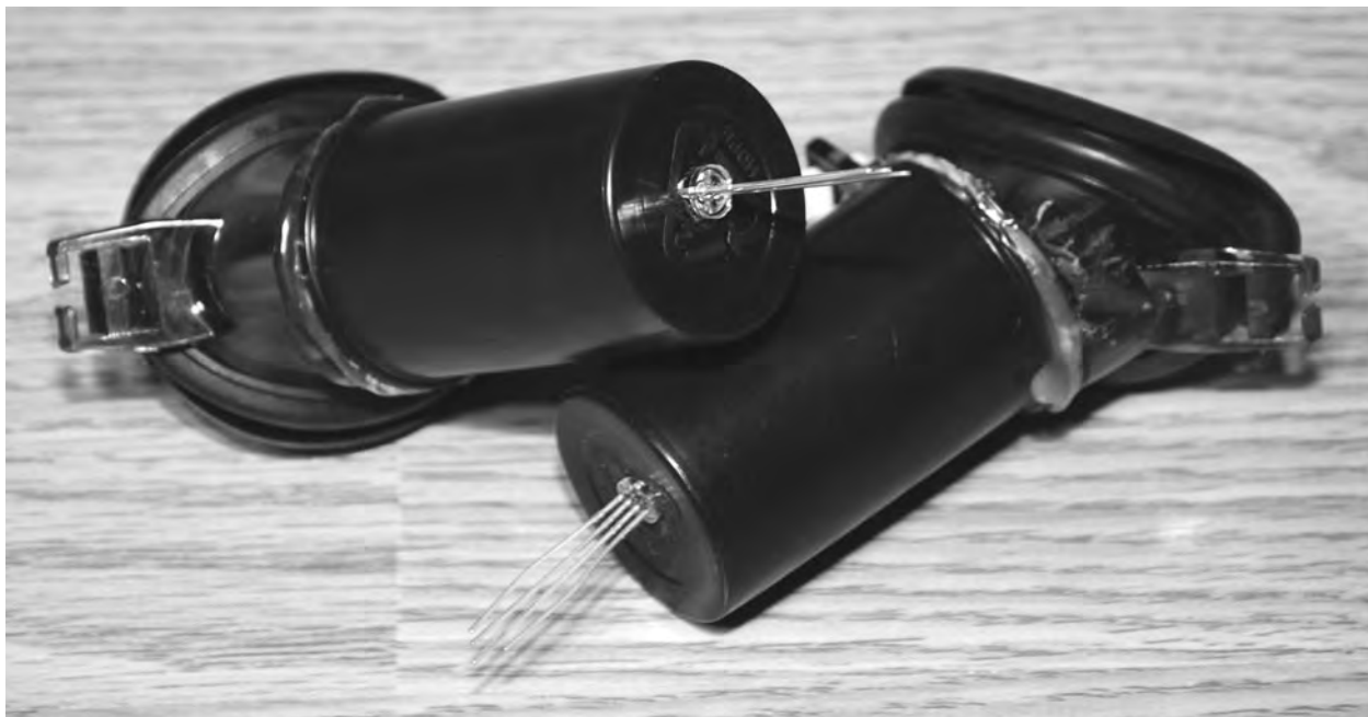
Figure 18-9 Diffuser tubes glued to the goggles.
