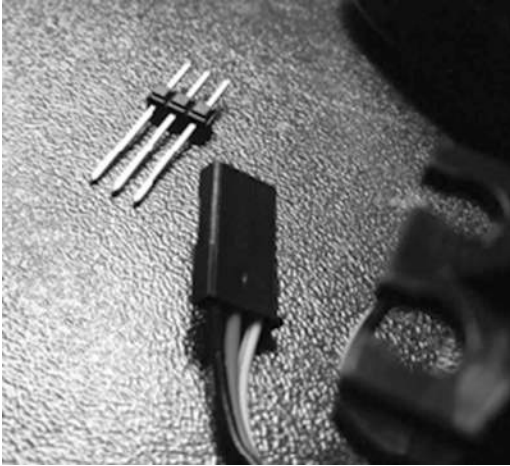
Figure 4-16. Header pins for servo motor connection
