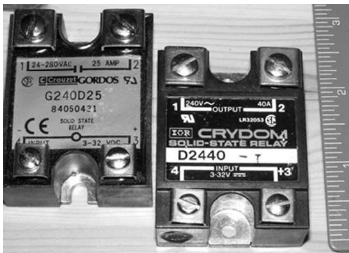
Figure 4-26. Two examples of a solid state relay
