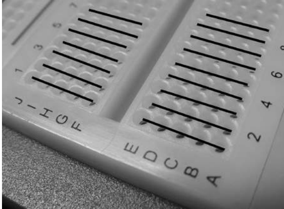
Figure C-2. Interconnected column holes
