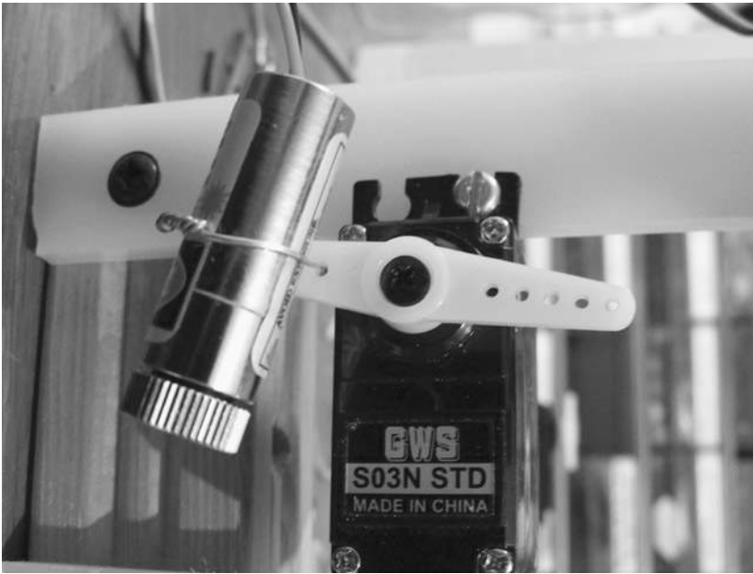
Figure 9-4. Laser diode mounted on servo motor
