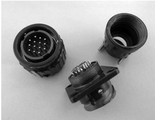
Figure 11-6. Disassembled plug and socket
