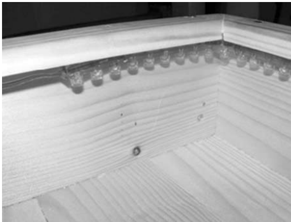
Figure 8-10. The compartment showing LED strip
