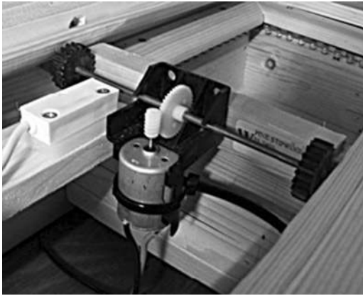
Figure 8-6. Panel drive assembly (with motor)
