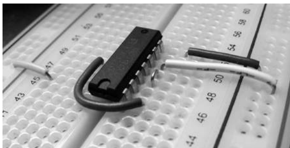
Figure C-7. Chip with power and signal jumpers installed
