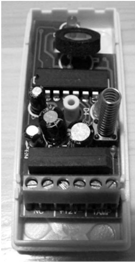
Figure 4-40. Inside the PIR sensor
