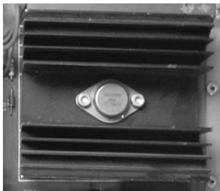
Figure 4-23. 2N3055 transistor on a heatsink
