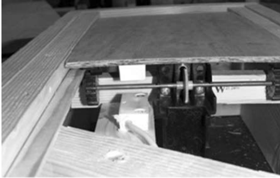
Figure 8-5. Panel drive assembly (without motor)
