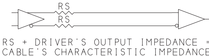
Figure 7-7: A series termination can absorb reflections.
