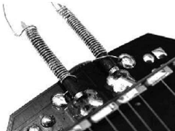
Finished sensor spring installation
