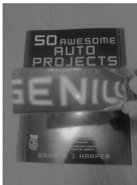
Figure 8-20 A thin Fresnel lens shown magnifying.
