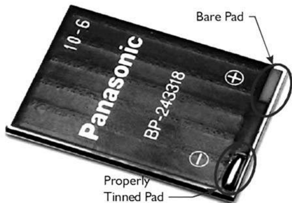
Figure 15-13 Step 8— assembling the Solarroller . Image courtesy Solarbotics.
