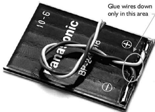
Figure 15-14 Step 9— assembling the Solarroller . Image courtesy Solarbotics.
