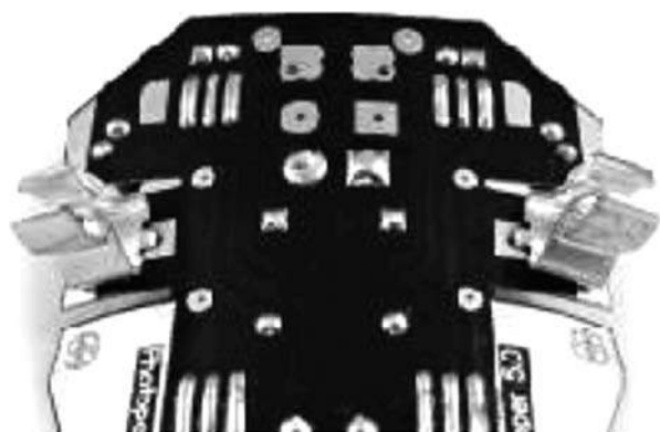
Figure 16-14 Both motor mounts ready. Image courtesy Solarbotics.
