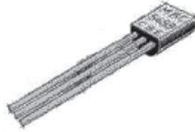
NPN transistor (PN100, BC548)
