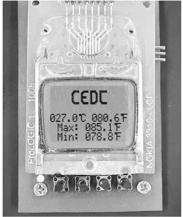
Figure 4-7 Temperature plotter display in readout mode
