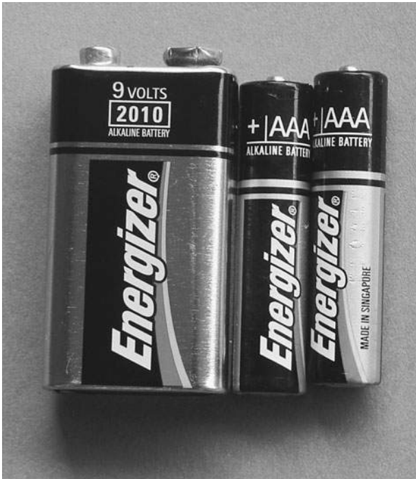
Figure 1-3 Alkaline battery in 9V- and AAA-size packages
