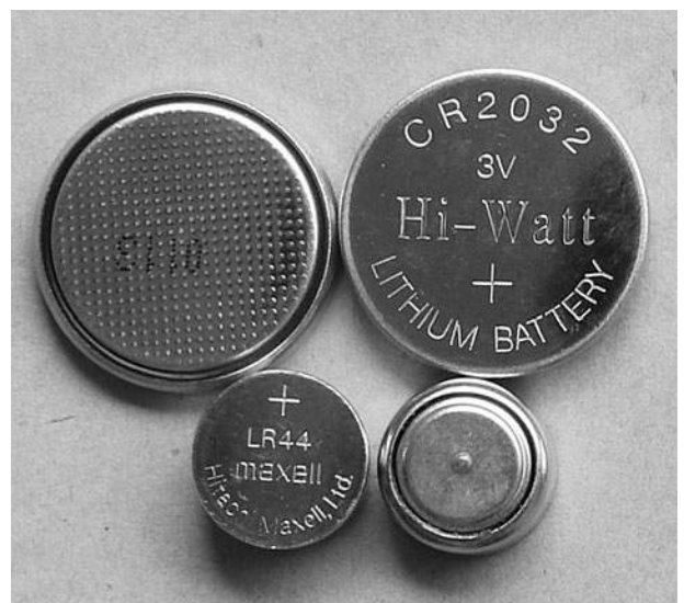
Figure 1-4 The smaller LR44 cell is an alkaline battery. The bigger CR2032 cell is a lithium battery.
